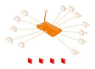
1. At least one rowter is required, as 16 directly connected EDs will exceed the maximum limit of 12. Four EDs will be orphaned.
