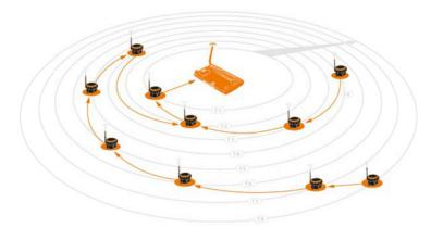
There can be a maximum depth of 8 layers of routers in a network amd a maximum of 200 nodes per metwork with the **RF-RXS** series of receivers.
