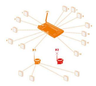
4. If either of the routers fail, the network can still be meaintained, as the 2 orphaned EDs can re-route via the other router.
