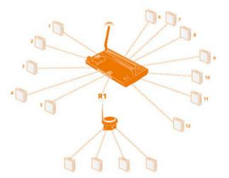
2. A single router (R1) will work, but gives no redundancy if the router should fail.
